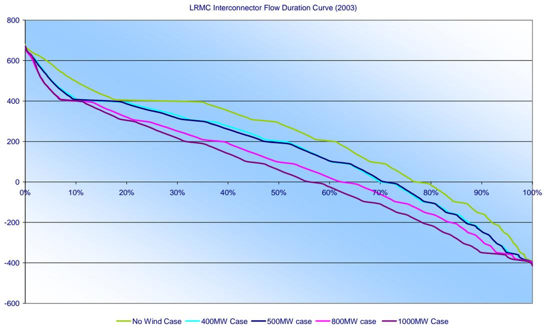
Figure 7-1 Interconnector Flow duration Curves for the LRMC analysis
