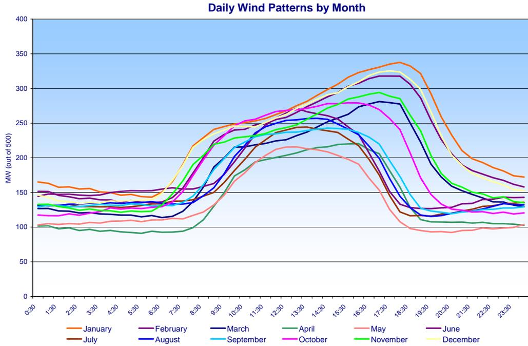
Figure 3-3 - Monthly Variation in Average Wind-farm Output (500MW case)
