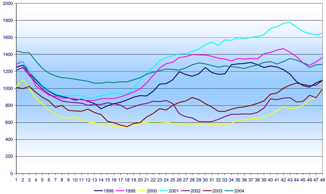
Figure 6-3 - January 1, SA Residual Electricity Demand after Wind generation has been removed (500 MW case)
