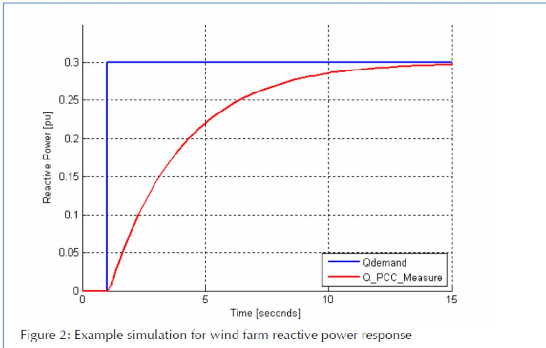
This example is a highly damped response and while a wind farm can be tuned to provide a slightly faster response it is unlikely that it could be produced within one second. This response however, is not the fast acting voltage support mechanism that occurs with low voltages. The reactive response that occurs for voltage support under fault conditions is much faster but this is a turbine by turbine response, not a “generating system” response.
