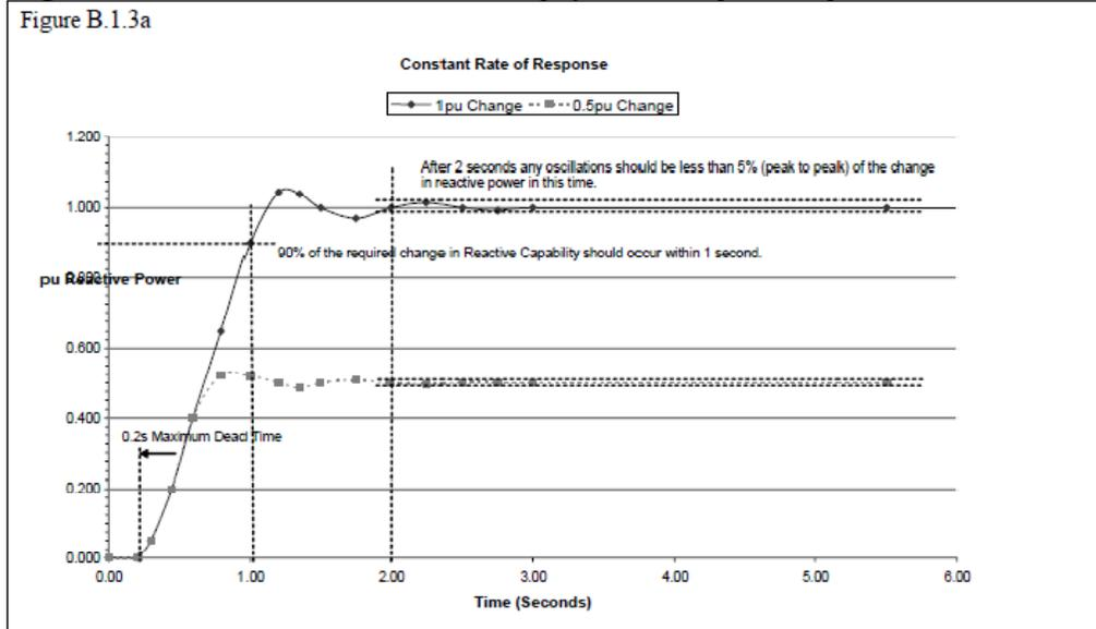
This clearly allows a dead band prior to the response commencing of 0.2 sec, and the requirement to reach 90% of the steady state response in 1 second. The proposed license drafting requires 'an initial response time of less than 200 msec' making the dead band less than 0.2 sec and the 'speed of response such that 95% of the steady state reactive power response is achieved within 1 second' is faster than the UK requirement of 90%.
