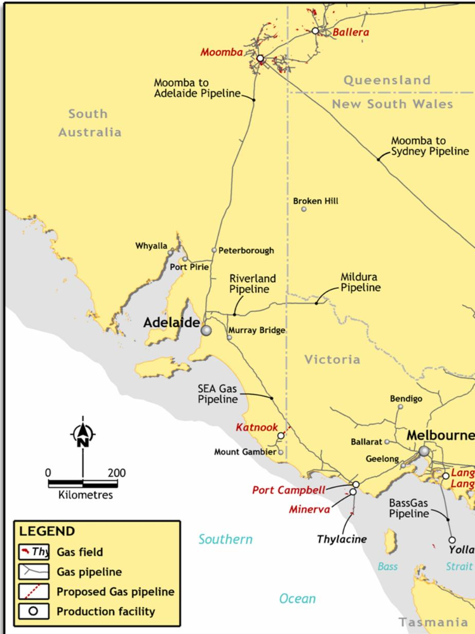
Source: Origin Energy. Note, Mount Gambier is now connected directly to the SEA Gas pipeline.
