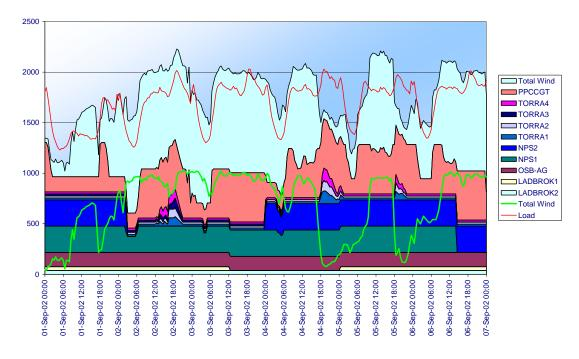
Figure 6-1- Example of Rapid Rate of Change of Wind-Farm Output (1,000 MW Case)
